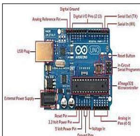
Fig.C.1: - Arduino Board
