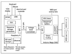
Fig. A.2: -Raspberry-Pi Architecture
